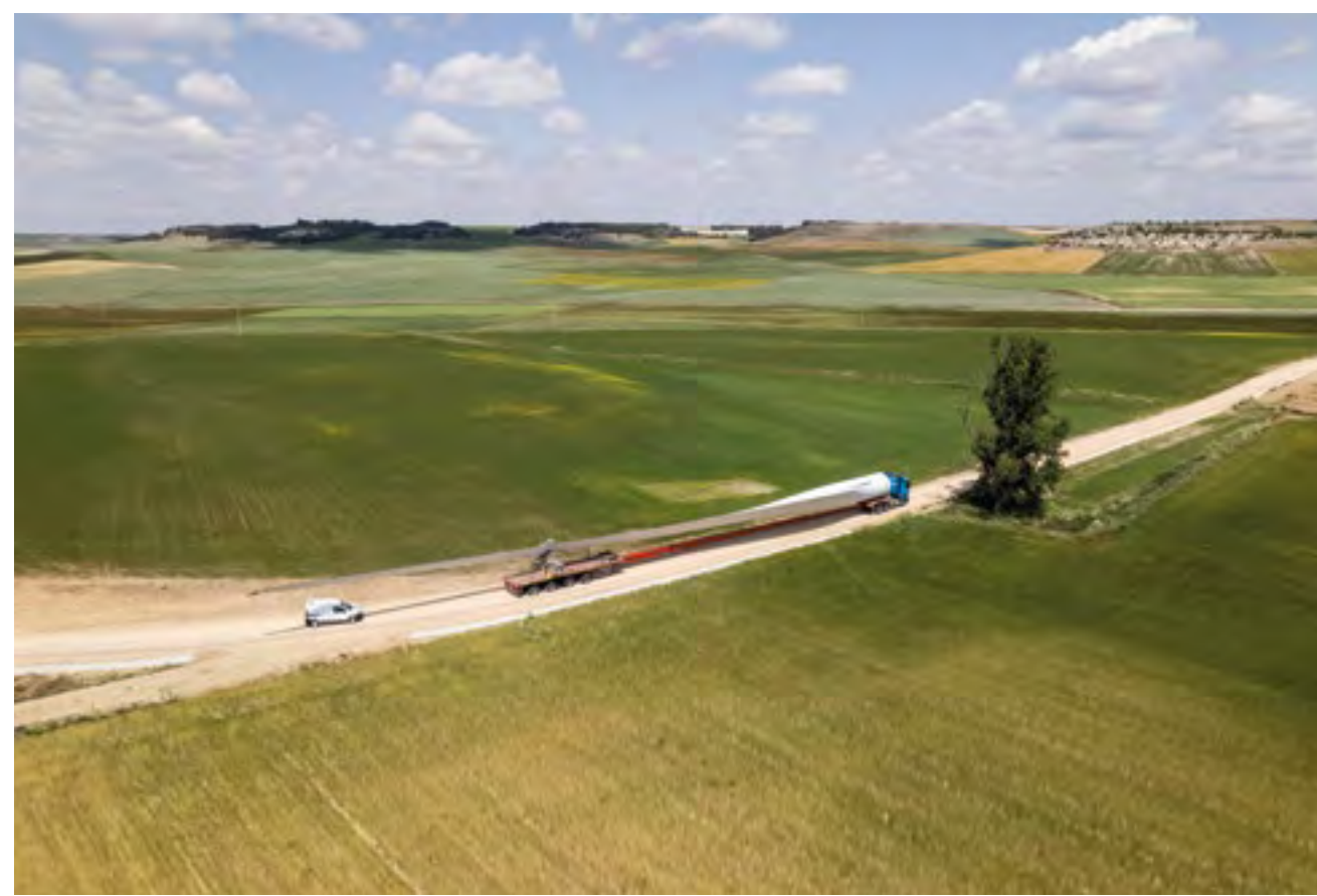
Transportation of large components, here the rotor blades
